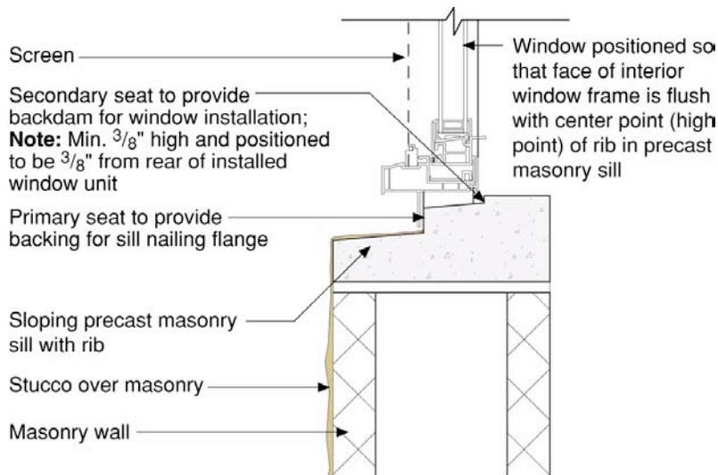
**Figure 8c: Window sill drainage section**
