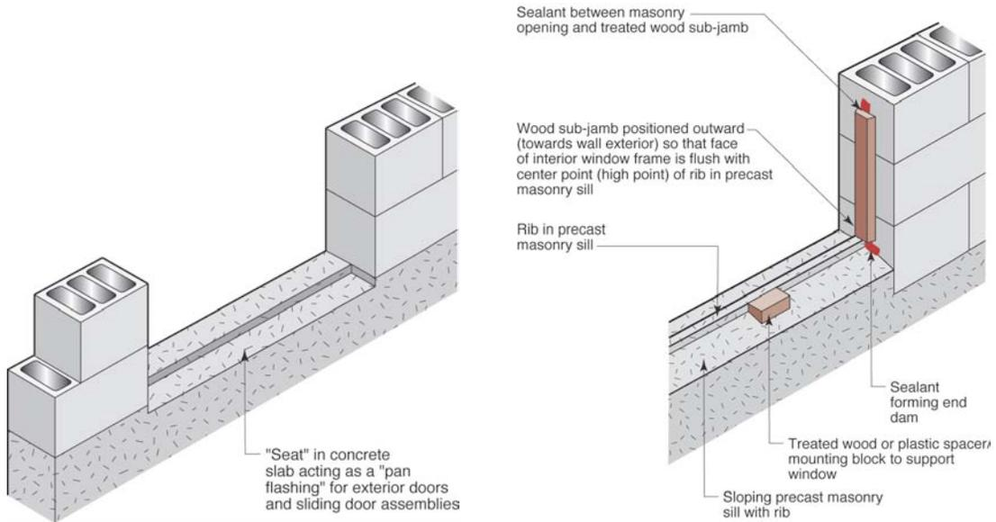
**Figure 8a: Exterior door pan flashing “seat”**
