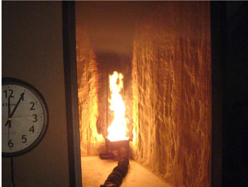
Test picture just prior to 160KW
